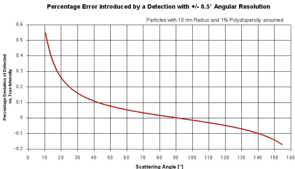
While the errors are still small enough to allow Molecular Weight Determination, exact determination of the Radius of Gyration becomes difficult to impossible for smaller particles - the systematic distortions due to the poor angular resolution can easily be of the same order as the slope of the intensity versus scattering angle for small particles !
