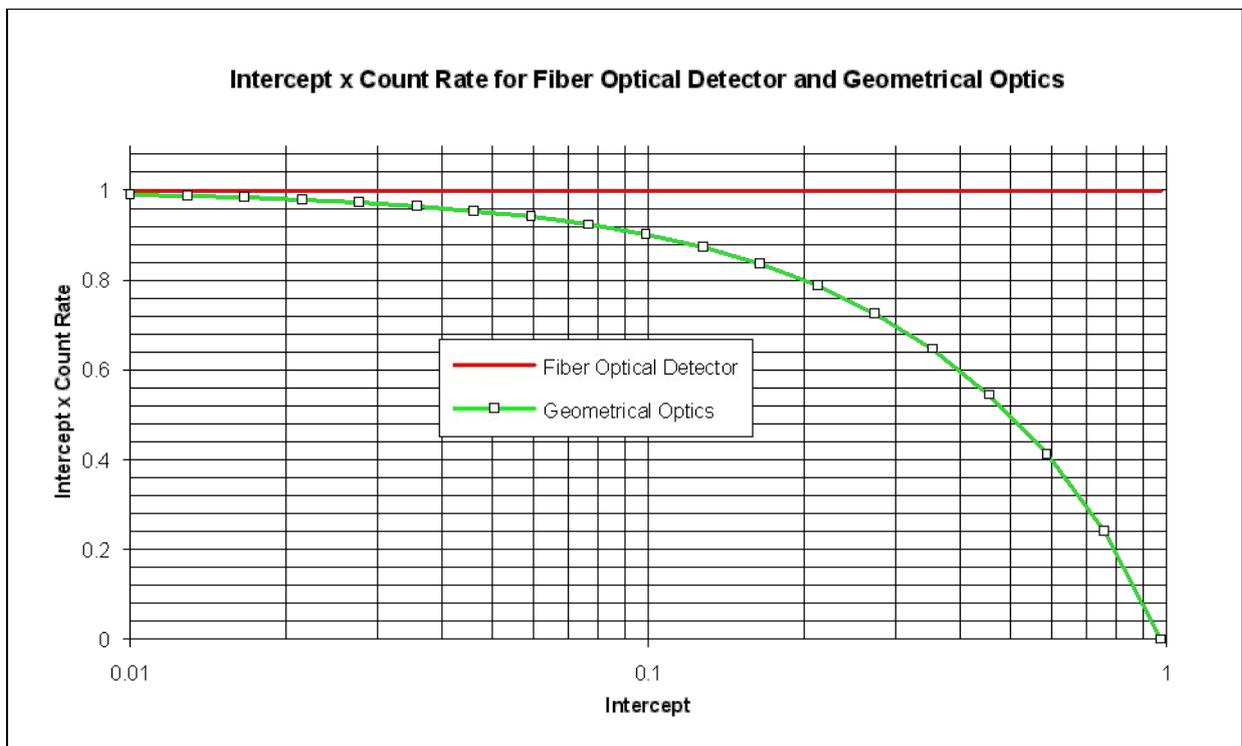
The above figure clearly shows the major disadvantage of using Geometrical Optics for detection - for high relative intercepts, which require a small number of modes ( $N_{Mode}$ ) or coherence areas to be detected only (-> **Coherent Detection**), the product of Intercept x Count Rate will drop dramatically, while it stays completely constant for the Fiber Optical Detection.
